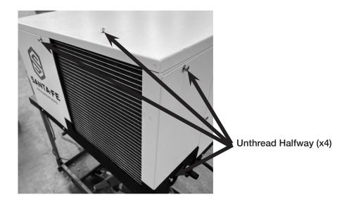
**Step 2:** Install supply duct plenum on the dehumidifier by slotting half-threaded screws in the keyed grooves (x4). Ensure screws are pushed all the way into the grooves.
