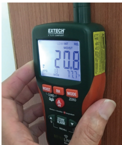
Wood moisture content of bookcase measured at a moist 20.8.
