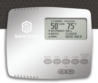
The RH will begin flashing, and can be adjusted up or down by pressing the set-point keys. By pressing program key again the Temperature will begin flashing. The temperature can be adjusted the same way. Pressing the program key again exits this mode. If no key is pressed for 5 seconds the control exits this mode.
