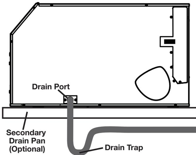
Note: The secondary drain pan is only needed if the dehumidifier is located above a living space.
